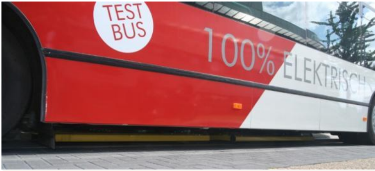
Caption: Automatic lowering of the pickup coils to the primary coil in the asphalt (Conductix-Wampfler)
