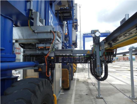
Caption: E-RTG with Drive-In L-Unit, connected to the conductor rail system
