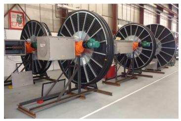
Caption: Motorized cable reels and special cables with a total length of over 1,000 meters for the supply of push carts for liquid iron and metal scrap.
