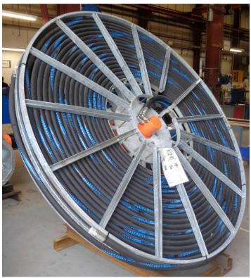
Caption: Hose reel with rotary transmitter and a 2  $\times$  1" connector for the supply of argon gas with two hoses
